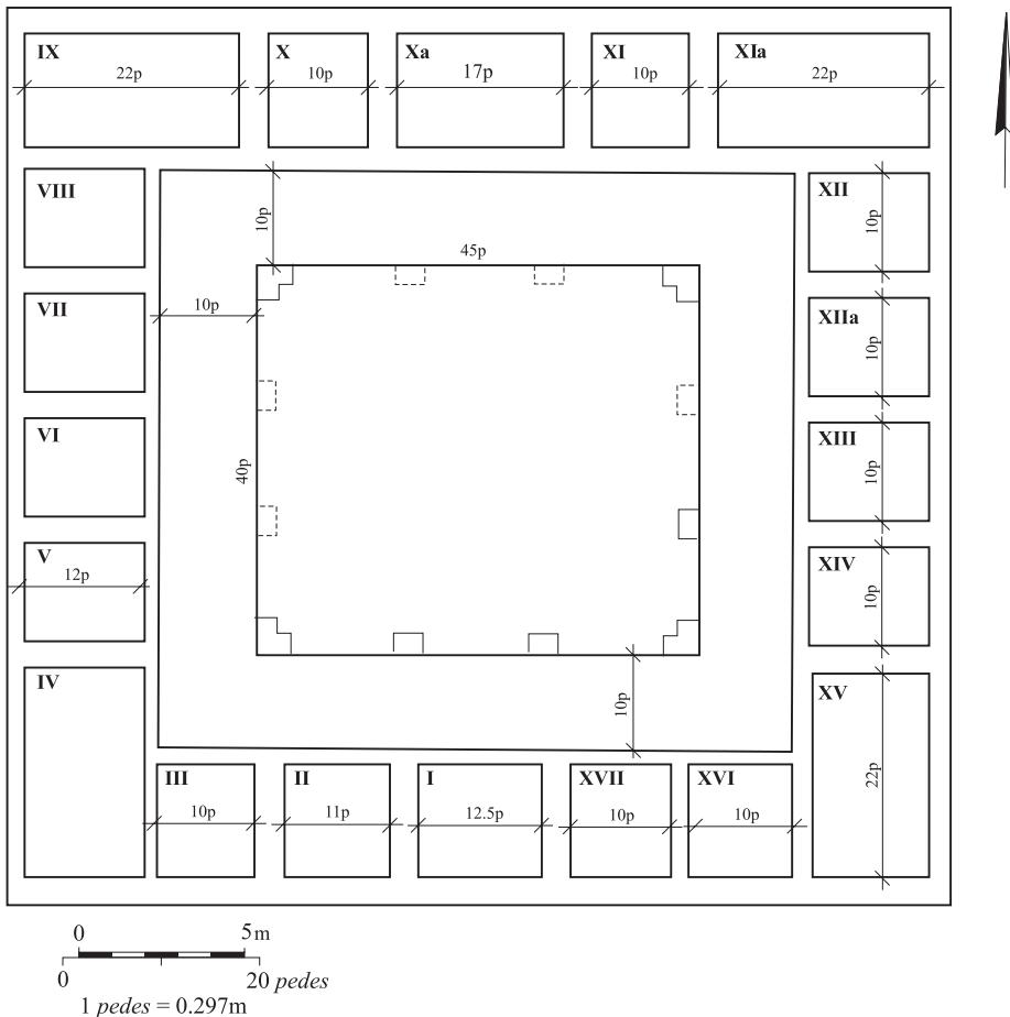
Fig. 1. A proposed plan showing rooms with dimensions in original *Pedes*.
